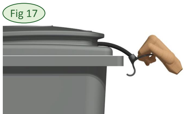
Fig. 16 & 17): And travel down towards the lifting comb of bin.
